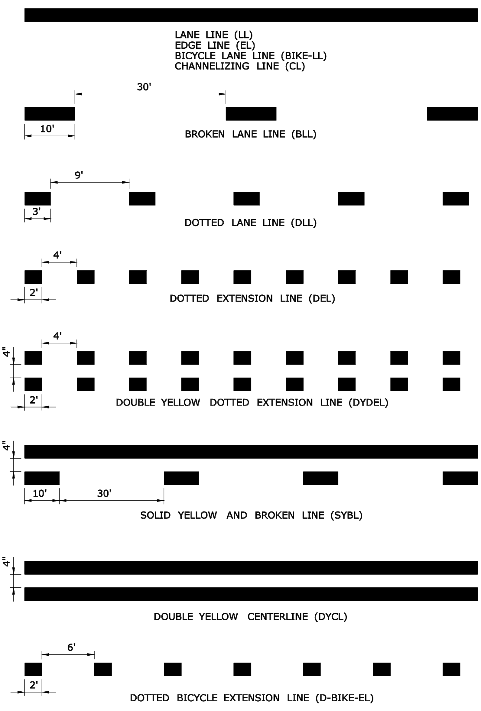
8.8 PAVEMENT MARKINGS TYPICAL DETAILS NTS
