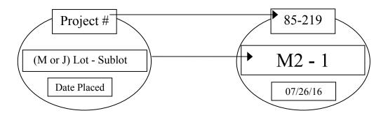
FIGURE 4.06-10: Labeling of Cores
