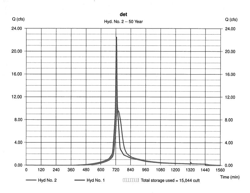
Hydraflow Hydrographs by Intelisolve v9.1
