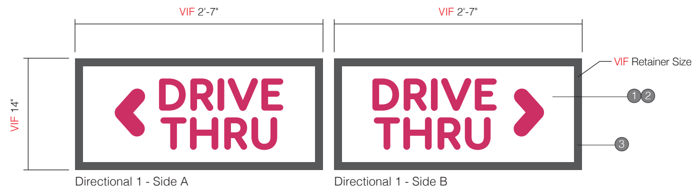
A Sign Elevation - Front View Scale: 1" = 1'-0"
