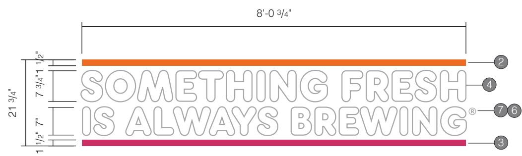
A Sign Elevation - Front View Scale: 1/2"=1'-0"
