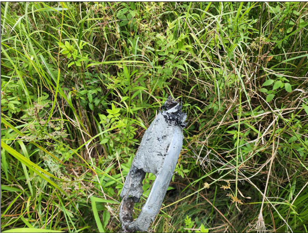
Photo 6: Sediment deposition above original deep organics (muck) soils was measured at each test hole (here Test Hole #2)
